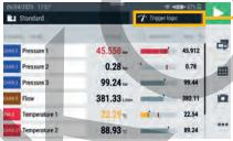
Numerical representation of 6 channels with bar graph Display of measuring range, warning and alarm values as well as MIN and MAX values
